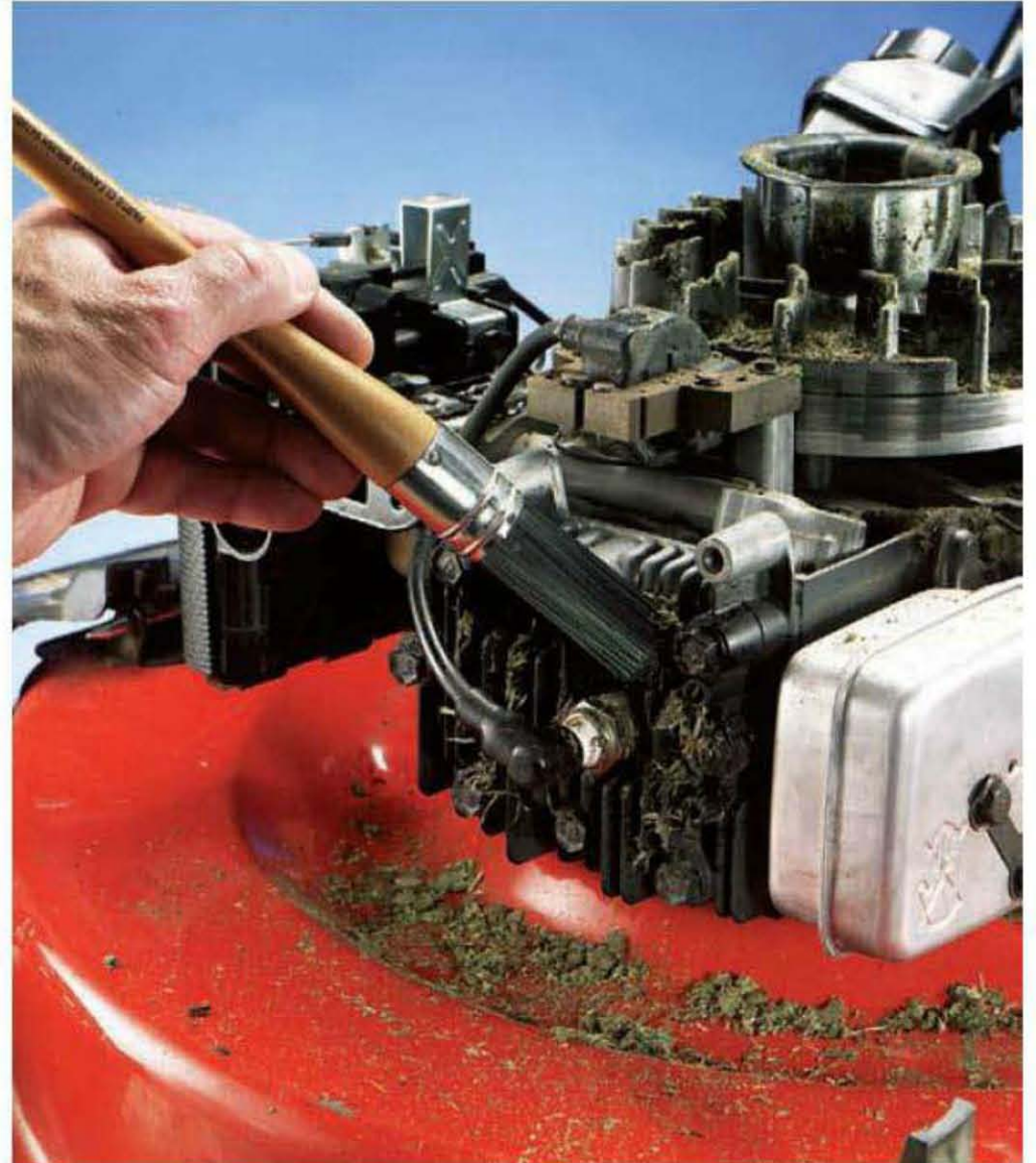
Use a stiff bristle brush to clean cooling fins and other engine parts after removing the blower housing.
