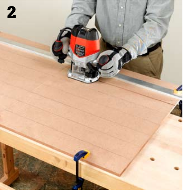
2 Clamp the MDF pieces to a bench with their faces up and their edges aligned. Using a router and a straightedge guide, mill a 3/16"-wide x 3/16"-deep groove into both pieces at each slot location. If the cabinet has a center partition (middle stile), cut the pieces in half so you'll be able to fit them into the cabinet.
