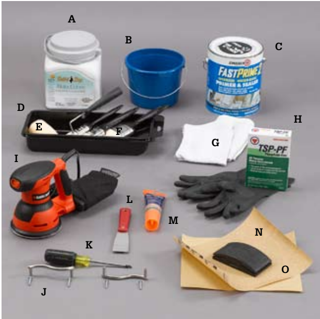
Tools and materials for painting wood cabinets include: (A) Semigloss or gloss enamel paint; (B) wash bucket; (C) primer; (D) roller tray; (E) roller sleeve (3"); (F) paintbrushes; (G) rags; (H) TSP cleaner and rubber gloves; (I) palm sander; (J) new cabinet hardware (optional); (K) screwdriver; (L) putty knife; (M) wood filler; (N) sandpaper (100- and 150-grit) and (O) sanding block.
