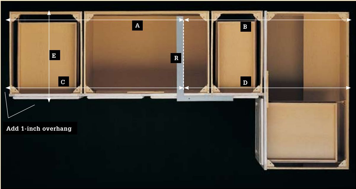
Measure along the tops of the base cabinets to determine the size of the countertop. If the wall corners are not square, use a framing square to establish a reference line (R) near the middle of the base cabinets, perpendicular to the front of the cabinets. Take four measurements (A, B, C, D) from the reference line to the cabinet ends. Allow for overhangs by adding 1" to the length for each exposed end and 1" to the width (E).
