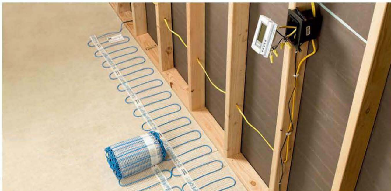
A radiant floor-warming system employs electric heating mats that are covered with floor tile to create a floor that's cozy under foot.
