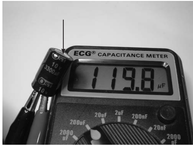
FIGURE 7-8 Bulging 3,300- \mu F electrolytic capacitor with greatly reduced capacitance.
