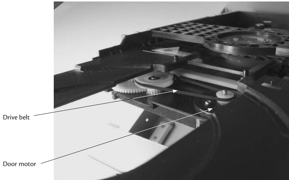
FIGURE 15-4 Door mechanism with belt on underside of platform. The leaf switch is not visible.
