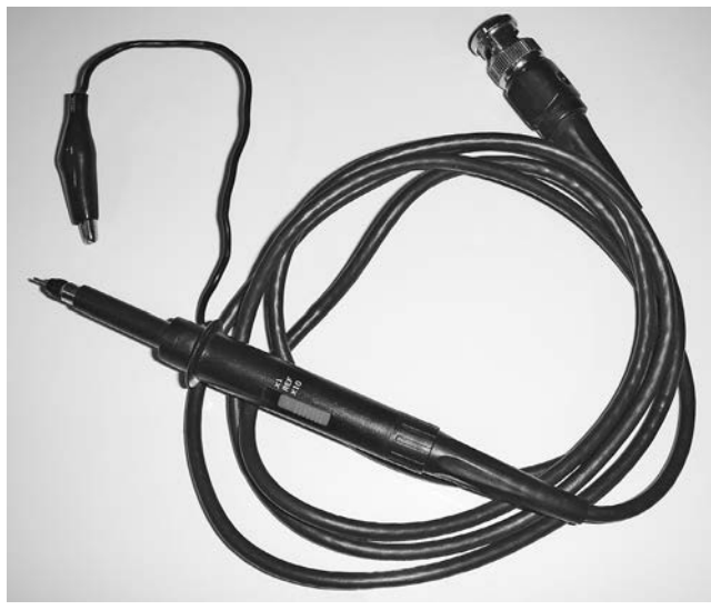
FIGURE 2-11 Oscilloscope probe, 10X/1X switchable.
