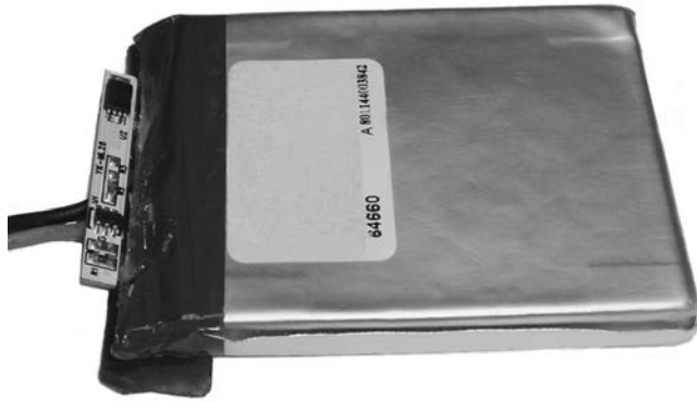
FIGURE 7-6 Lithium battery with BMS board.
