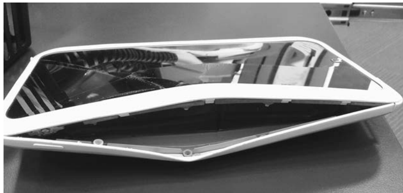
FIGURE 14-8 E-reader destroyed by a swollen battery. Look how big it got!
