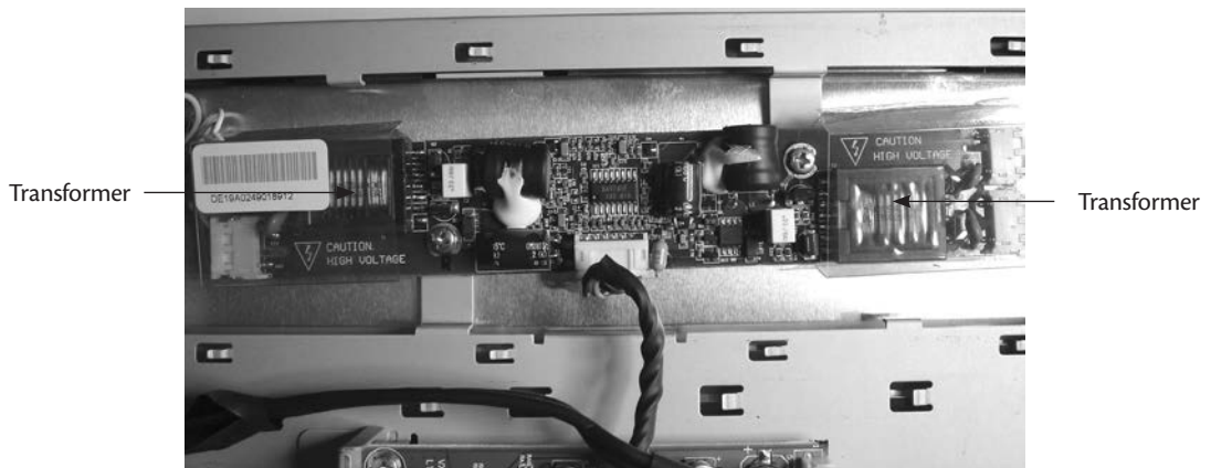
FIGURE 10-5 LCD backlight inverter. Note the plastic insulation over the transformers.
