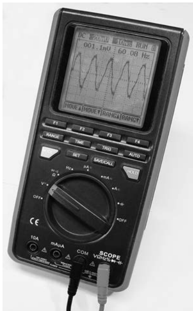
FIGURE 2-9 Scopemeter with banana plug input.
