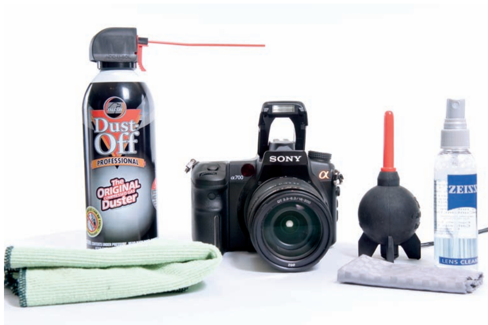
AA.6 The A700 with the basic cleaning tools: Compressed air, a Giotto's Rocket Air Blaster, Zeiss lens-cleaner solution, a microfiber cleaning cloth, and a lint-free cleaning cloth.
