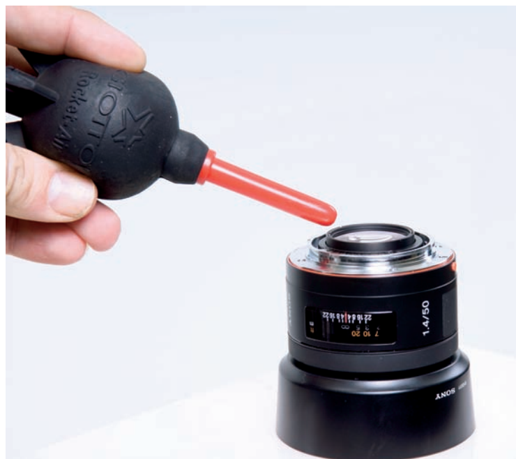
AA.4 Giotto's Rocket Air Blaster is a great tool for removing dust and dirt from the lens. Here one is being used to gently blow the dust and dirt from the rear element of a lens.
