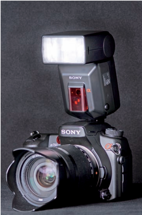
4.11 A dedicated flash unit can be set at various angles when mounted on the camera.
