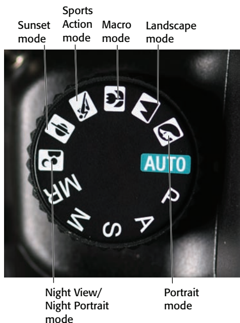
1.29 The Mode dial makes it easy to quickly switch Scene Exposure modes.
