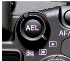
1.27 The Metering mode lever makes it easy to switch among Metering modes.
