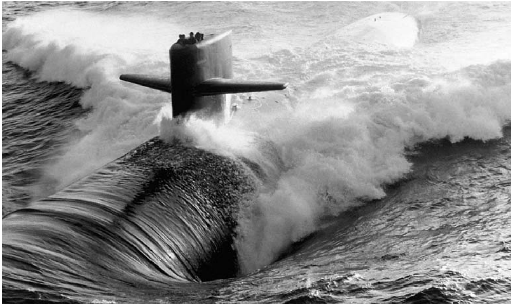
When a submarine needs to come to the surface, compressed air is blown into its ballast tanks.
