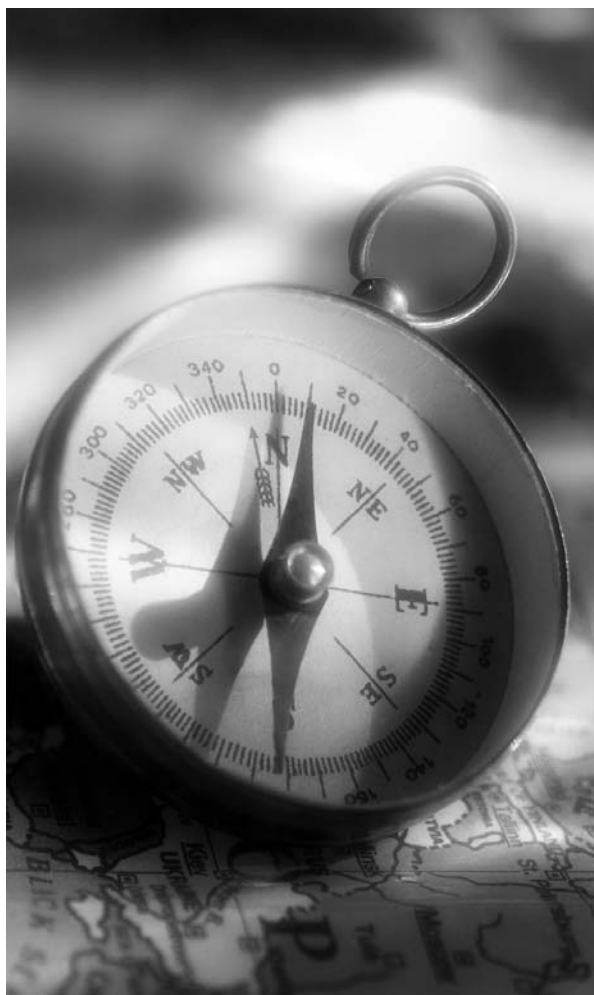
The needle of a compass is actually a magnet, and it will always point toward Earth's magnetic North Pole.
